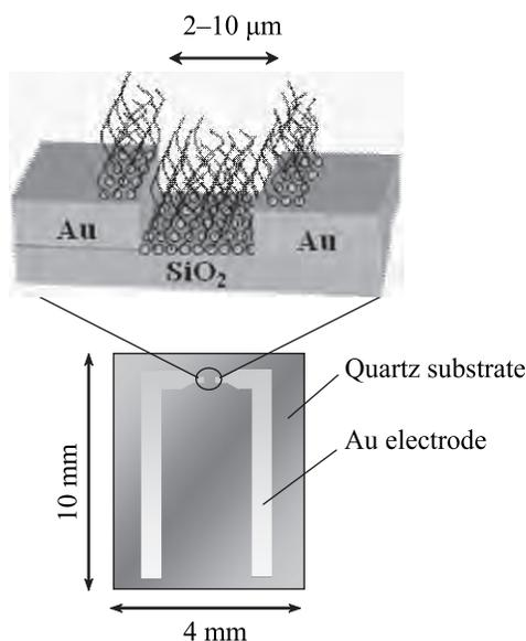
Fig. 1. Schematic diagram of MWNT-based sensor.
