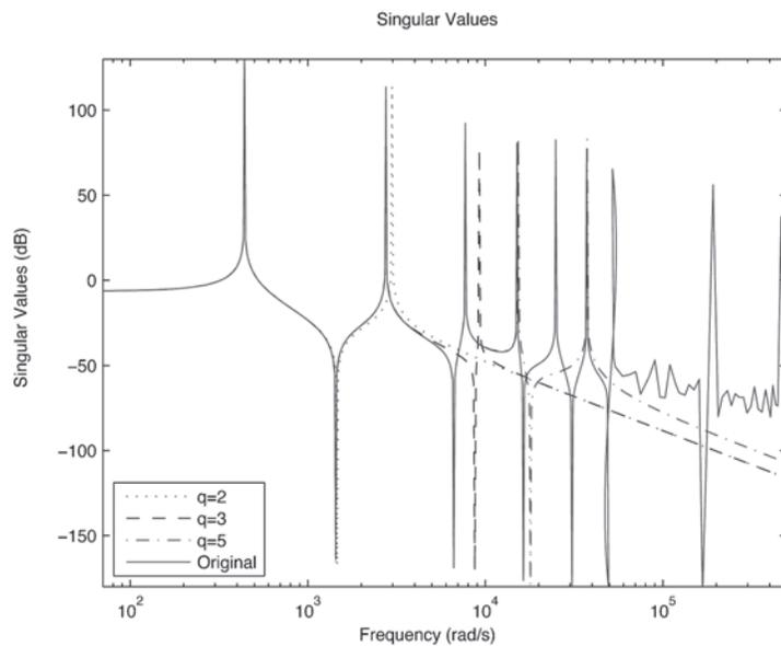
Fig. 2. Frequency response of the reduced systems of the undamped model.
