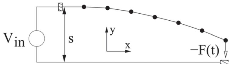
Fig. 1. Conducting clamped beam with counter electrode below right end.
