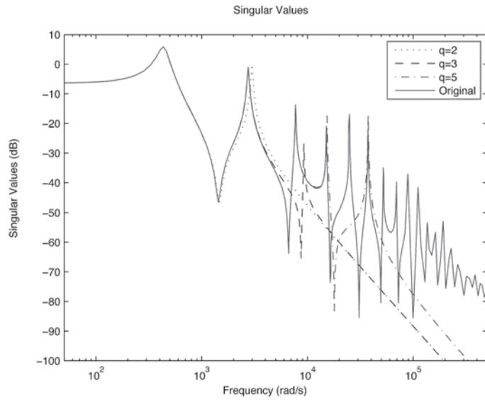
Fig. 4. Frequency response of the reduced systems of the damped model.
