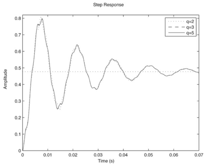
Fig. 5. Step response of the reduced systems of the damped model.
