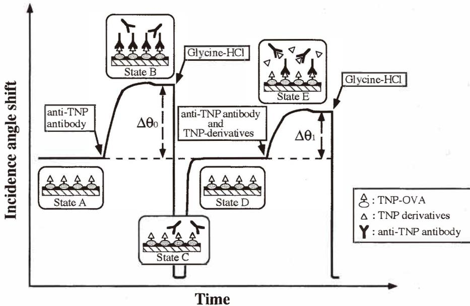
Fig. 1. Response transients of the TNP-OVA immobilized sensor to the anti-TNP antibody without antigen ( $\Delta\theta_0$ ) and with antigen ( $\Delta\theta_1$ ).
