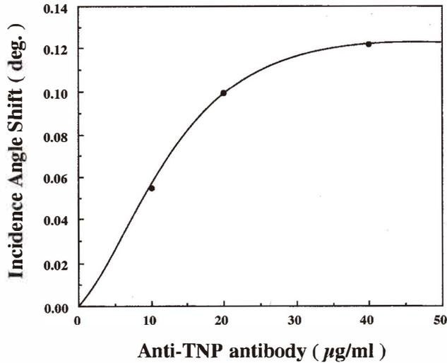
Fig. 5. Dependence of anti-TNP antibody concentration on the incidence angle shift of the TNP-OVA immobilized sensor.
