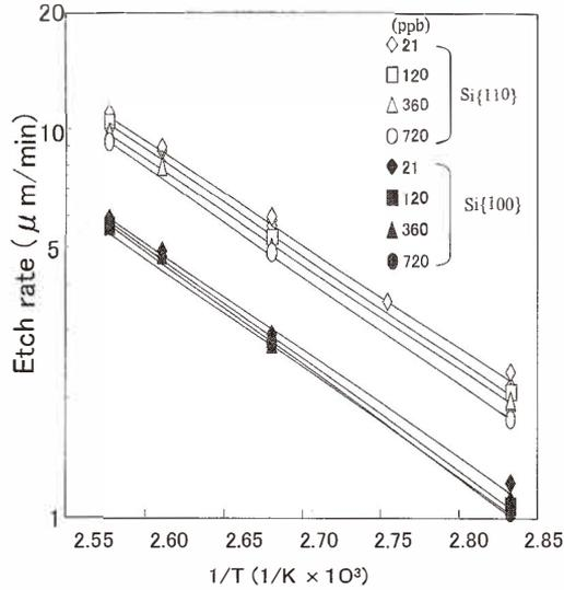
Fig. 3. Dependence of the Si{110} and {100} etch rates in KOH solution containing ppb-level of Cu on temperature (32wt% KOH).
