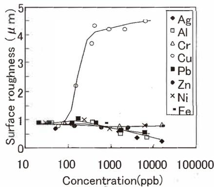
Fig. 7. Dependence of the surface roughness of Si{110} plane on concentration of impurities (32wt% KOH, 110°C).
