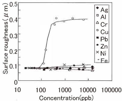
Fig. 8. Dependence of the surface roughness of Si{100} plane on concentration of impurities (32wt% KOH, 110°C).
