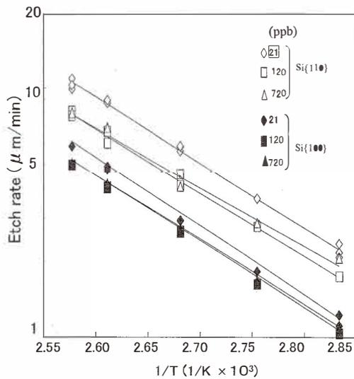
Fig. 4. Dependence of the Si{110} and {100} etch rates in KOH solution containing ppb-level of Pb on temperature (32wt% KOH).
