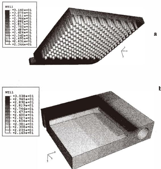
Fig. 7. Temperature distributions across the section and the bottom surface of the pin-fin sink (a) and across the section and the top surface of the channeling box (b).
