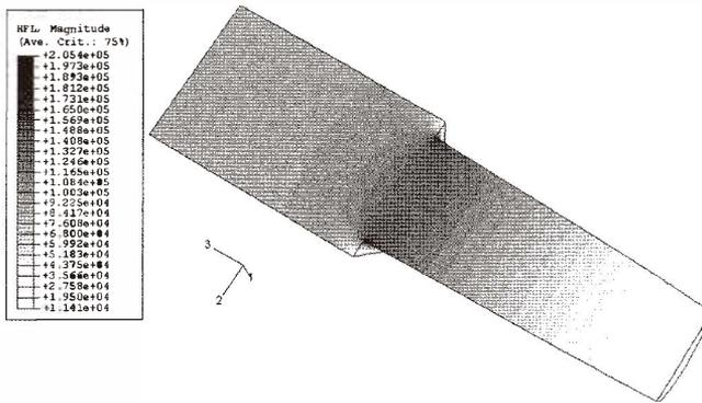
Fig. 14. Heat flux magnitude distribution across the cross-section of the simple model.
