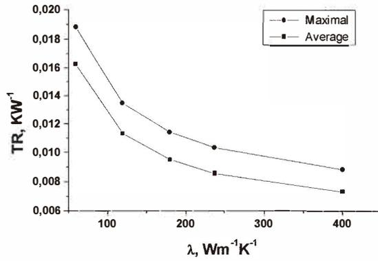
Fig. 9. Converter thermal resistance as a function of pin-fin sink material thermal conductivity.
