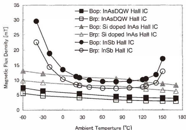
Fig. 6. Temperature dependence of the operation magnetic field of various types of hybrid Hall ICs.
