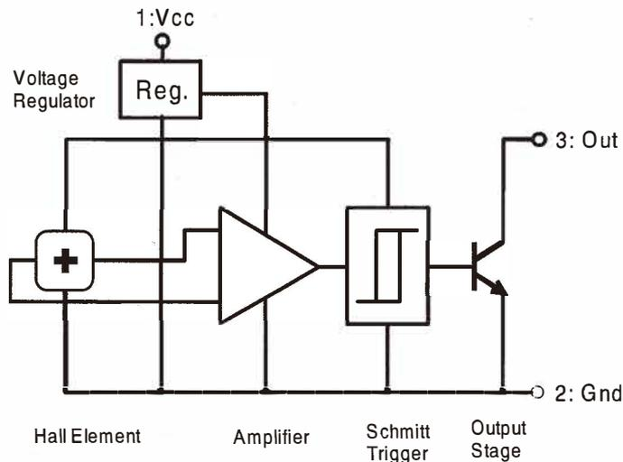
Fig. 1. Schematic diagram of hybrid Hall IC.
