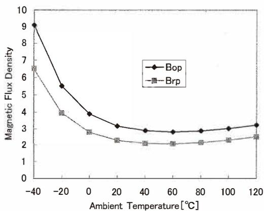
Fig. 4. Temperature dependence of the operation magnetic field of hybrid InSb thin film Hall IC.
