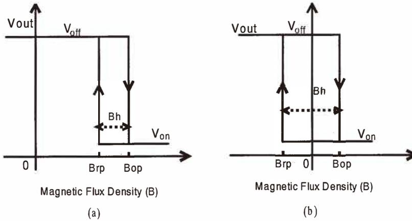
Fig. 2. Operational characteristics with hysteresis loop of hybrid Hall IC.
