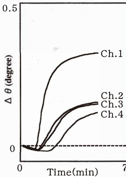
Fig. 7. Typical responses of each channel (Ch. 1–Ch. 4) of the SPR sensor to a *moromi* sample fermented for 14 days, where diluted ammonia was used as the reference liquid.
