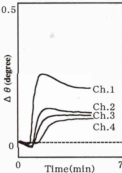
Fig. 4. Typical responses of each channel (Ch. 1-Ch. 4) of the SPR sensor to a *moromi* sample fermented for 14 days, where distilled water was used as the reference liquid.
