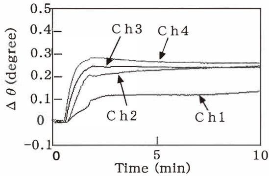
Fig. 12. Typical responses of each channel (Ch. 1–Ch. 4) of the SPR sensor to the *Yamahai-ginzyou* sample, where distilled water was used as the reference liquid.
