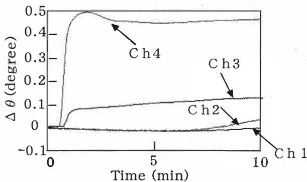
Fig. 9. Typical responses of each channel (Ch. 1–Ch. 4) of the SPR sensor to the *Gin-kouburi* sample, where distilled water was used as the reference liquid.
