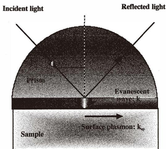
Fig. 1. Kretschmann-type SPR configuration.
