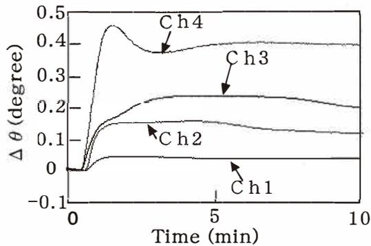
Fig. 15. Typical responses of each channel (Ch. 1–Ch. 4) of the SPR sensor to the *Tokuzyou* sample, where distilled water was used as the reference liquid.
