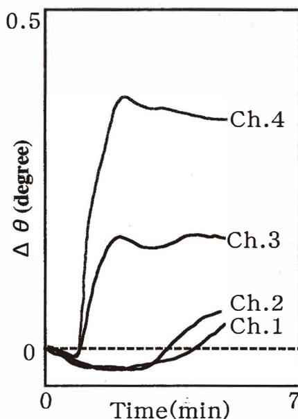
Fig. 5. Typical responses of each channel (Ch. 1–Ch. 4) of the SPR sensor to a *moromi* sample fermented for 23 days, where distilled water was used as the reference liquid.
