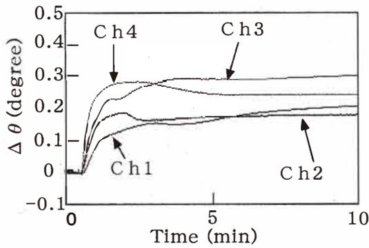
Fig. 13. Typical responses of each channel (Ch. 1–Ch. 4) of the SPR sensor to the *Yamahai-zyunmai* sample, where distilled water was used as the reference liquid.
