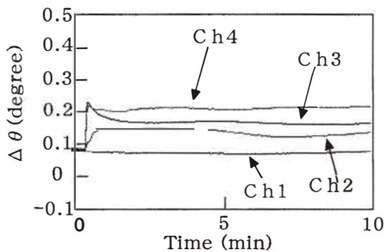
Fig. 11. Typical responses of each channel (Ch. 1–Ch. 4) of the SPR sensor to the *Bunsei-rokunen* sample, where distilled water was used as the reference liquid.
