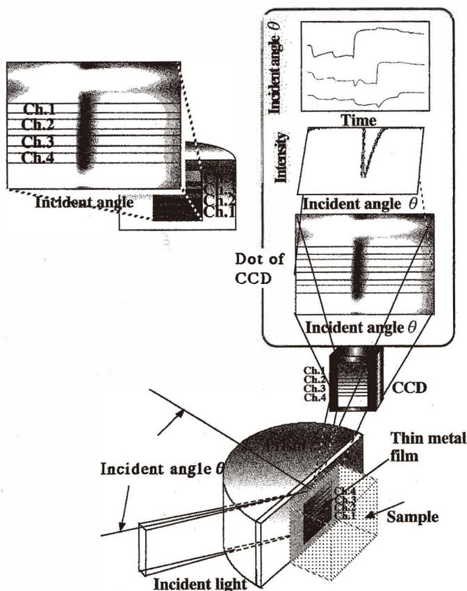
Fig. 2. Schematic diagram of the SPR sensor system.
