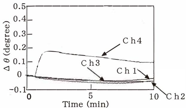
Fig. 10. Typical responses of each channel (Ch. 1–Ch. 4) of the SPR sensor to the *Kokosyu-ginzyou* sample, where distilled water was used as the reference liquid.
