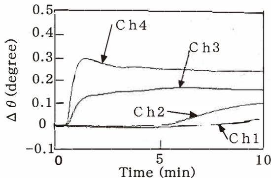
Fig. 16. Typical responses of each channel (Ch. 1–Ch. 4) of the SPR sensor to the *Taka* sample, where distilled water was used as the reference liquid.
