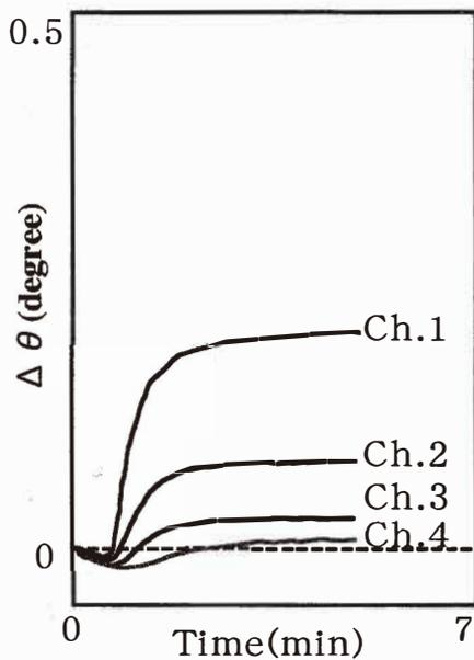
Fig. 3. Typical responses of each channel (Ch. 1-Ch. 4) of the SPR sensor to a *moromi* sample fermented for 5 days, where distilled water was used as the reference liquid.
