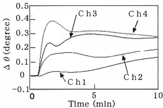
Fig. 14. Typical responses of each channel (Ch. 1–Ch. 4) of the SPR sensor to the *Yawara* sample, where distilled water was used as the reference liquid.
