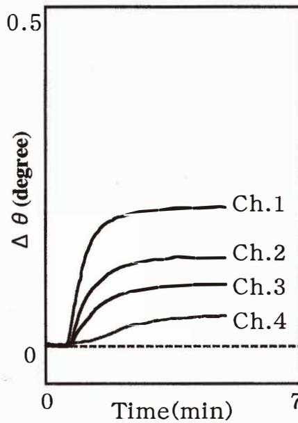
Fig. 6. Typical responses of each channel (Ch.1–Ch.4) of the SPR sensor to a *moromi* sample fermented for 5 days, where diluted ammonia was used as the reference liquid.
