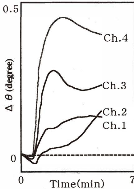
Fig. 8. Typical responses of each channel (Ch. 1–Ch. 4) of the SPR sensor to a *moromi* sample fermented for 23 days, where diluted ammonia was used as the reference liquid.
