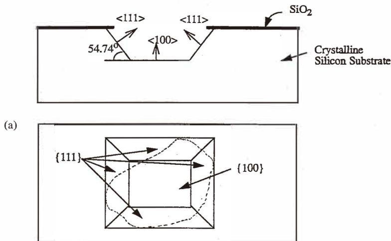
Fig. 1. (a) Cross-sectional and top view schematics of the etching of  $\{100\}$  Si having an arbitrarily shaped concave mask opening. The dashed line indicates the edge of the opening in the masking oxide. The etch exposes slow etching planes, such that the final structure is bounded by a rectangle circumscribing the mask opening.
