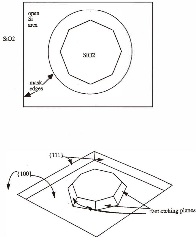
Fig. 1. (b) Top and perspective view schematics of the etching of  $\{100\}$  Si having a circular convex mask shape inside a concave square. Fast etching planes are exposed by the convex features, while slow etching  $\{111\}$  planes are exposed by the concave features. The masking oxide is not shown in the perspective view.
