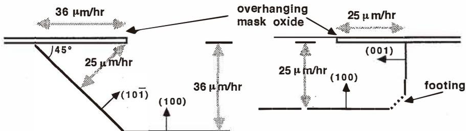
Fig. 3. Schematic of cross section of under-etched inclined planes at  $\delta = 0^\circ$ . At left is a 45°-inclined {110} plane, while at right is a vertical {100} plane, with a small  $\sim$ {110} footing.
