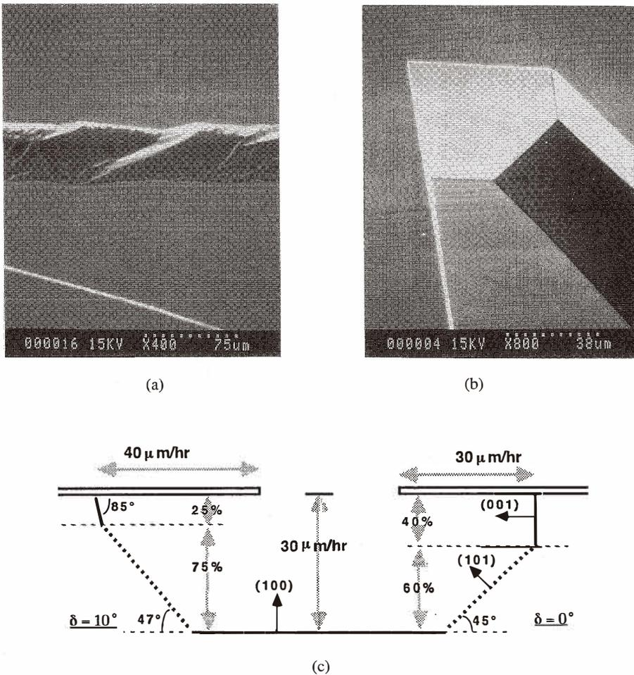
Fig. 4. Scanning electron micrographs of  $\langle 100 \rangle$  wafer after under-etch experiment in TMAH 21.2%, and subsequent removal of masking oxide: (a) showing the very rough side of the etched pit of the triangle at  $\delta = 27^\circ$ ; (b) showing (at the right side of the picture) the two-faceted side of an etch pit having  $\delta \sim 0^\circ$ . (c) Schematic showing the two facets of under-etched planes etched in TMAH 21.2% without IPA.
