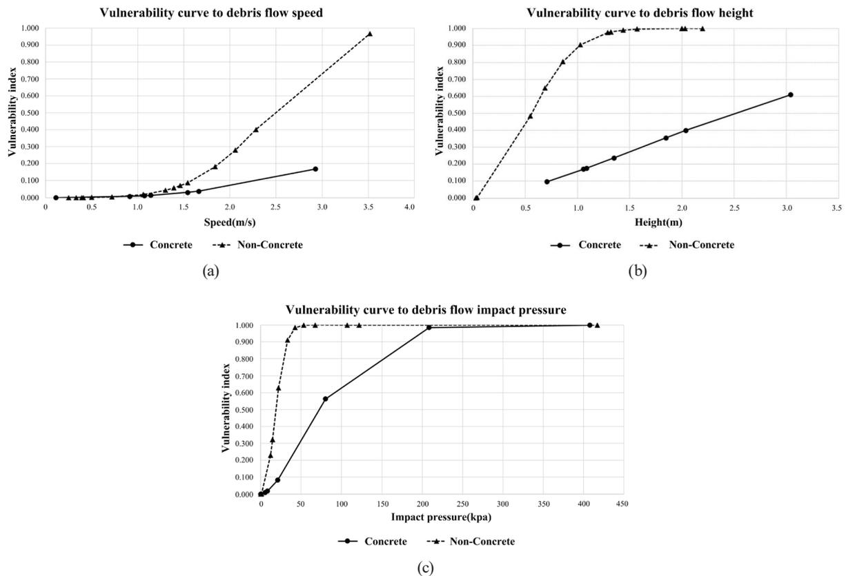
Fig. 6. Building vulnerability curve for different debris flow characteristics (watershed 1, 200-year frequency). (a) Debris flow speed, (b) debris flow height, and (c) debris flow impact pressure.
