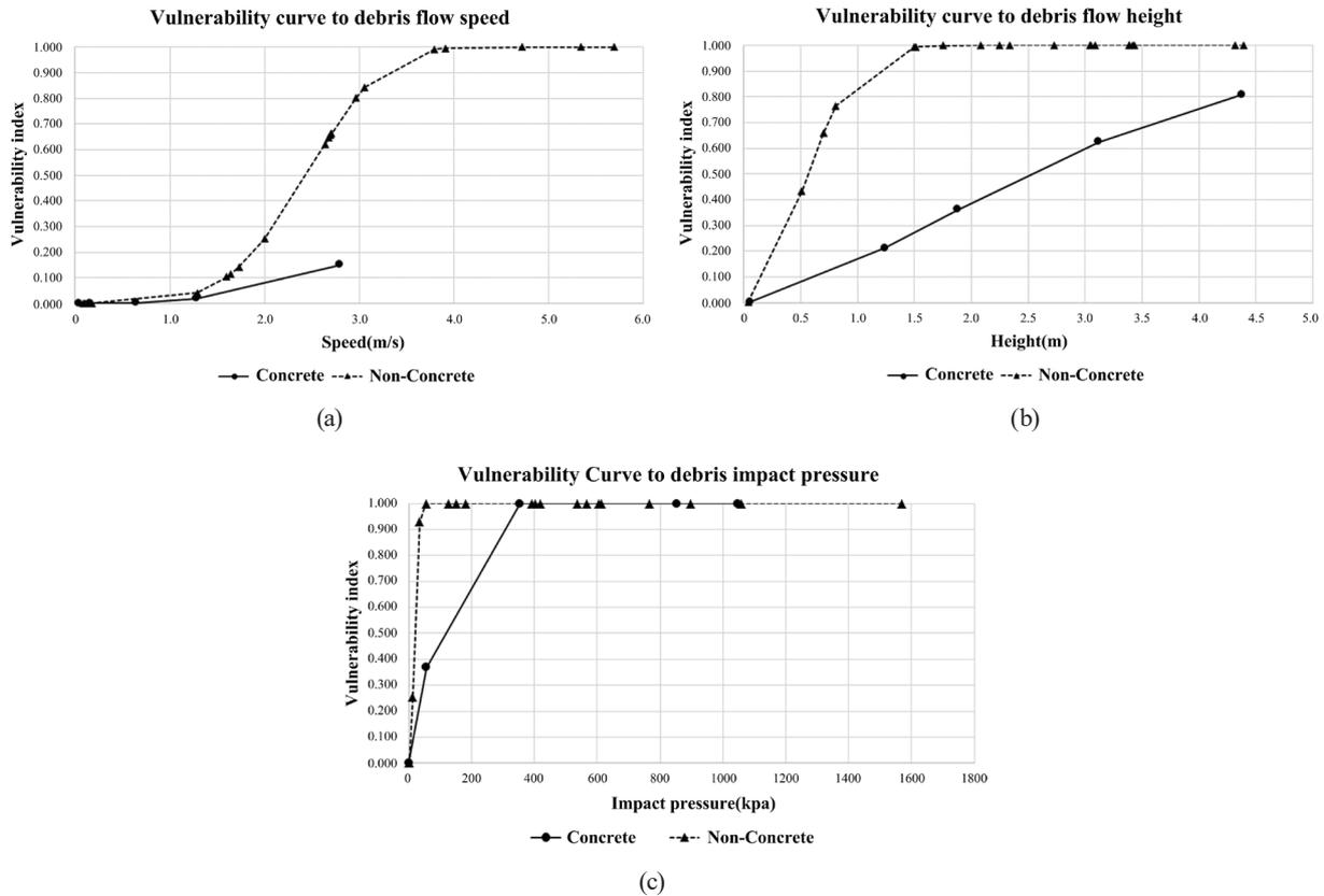
Fig. 7. Building vulnerability curve for different debris flow characteristics (watershed 2, 200-year frequency). (a) Debris flow speed, (b) debris flow height, and (c) debris flow impact pressure.
