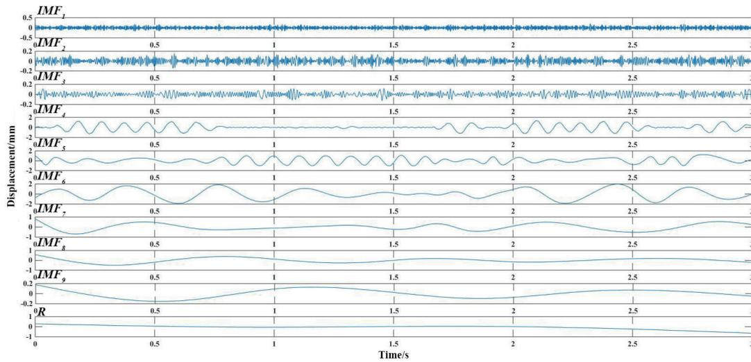
Fig. 3. (Color online) Decomposed IMFs of analog signal  $Y(t)$  obtained by ESMD.
