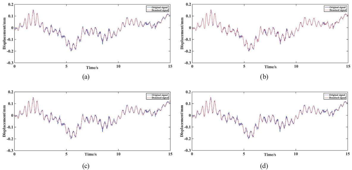
Fig. 10. (Color online) Comparison between denoised signals obtained by four denoising methods and original signal. Original and denoised signals obtained by (a) SVD, (b) ESMD, (c) SVD-EEMD, and (d) ESMD-SVD.
