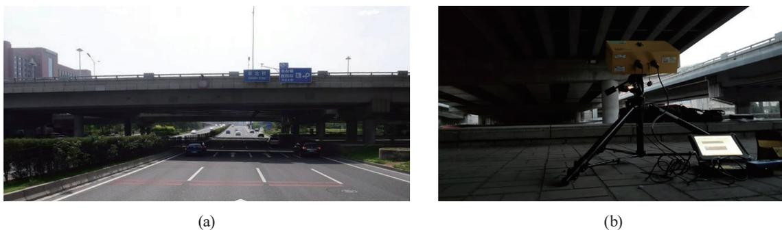
Fig. 6. (Color online) Fengbei Bridge and IBIS-S layout. (a) Fengbei Bridge and (b) dynamic deflection measurement of Fengbei Bridge using IBIS-S.
