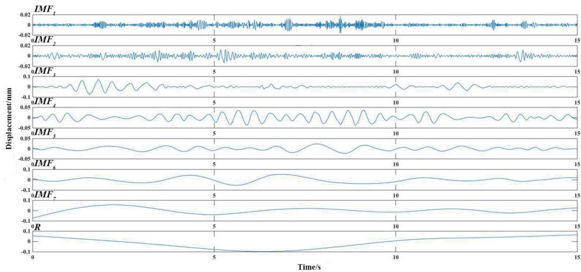
Fig. 8. (Color online) Decomposed IMFs of original bridge signal obtained by ESMD.
