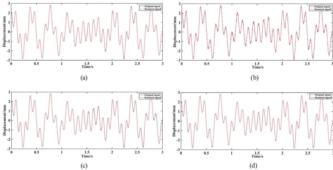
Fig. 5. (Color online) Comparisons of curves of signal  $X(t)$  and denoised signals obtained by SVD, ESMD, EEMD-SVD, and ESMD-SVD. (a)  $X(t)$  and signal denoised by SVD, (b)  $X(t)$  and signal denoised by ESMD, (c)  $X(t)$  and signal denoised by EEMD-SVD, and (d)  $X(t)$  and  $Y^*(t)$ .
