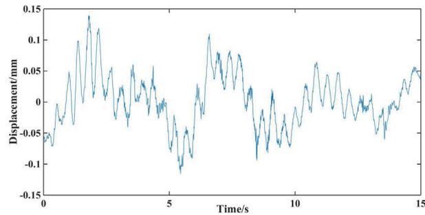
Fig. 7. (Color online) Waveform of signal of Fengbei Bridge obtained using IBIS-S.
