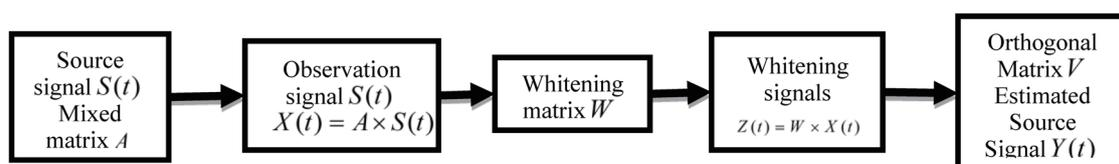
Fig. 3. Flow of SOBI signal processing.
