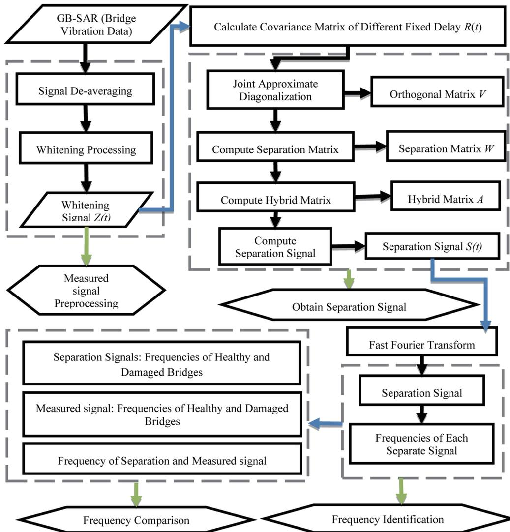
Fig. 4. (Color online) Flow of SOBI signal processing.
