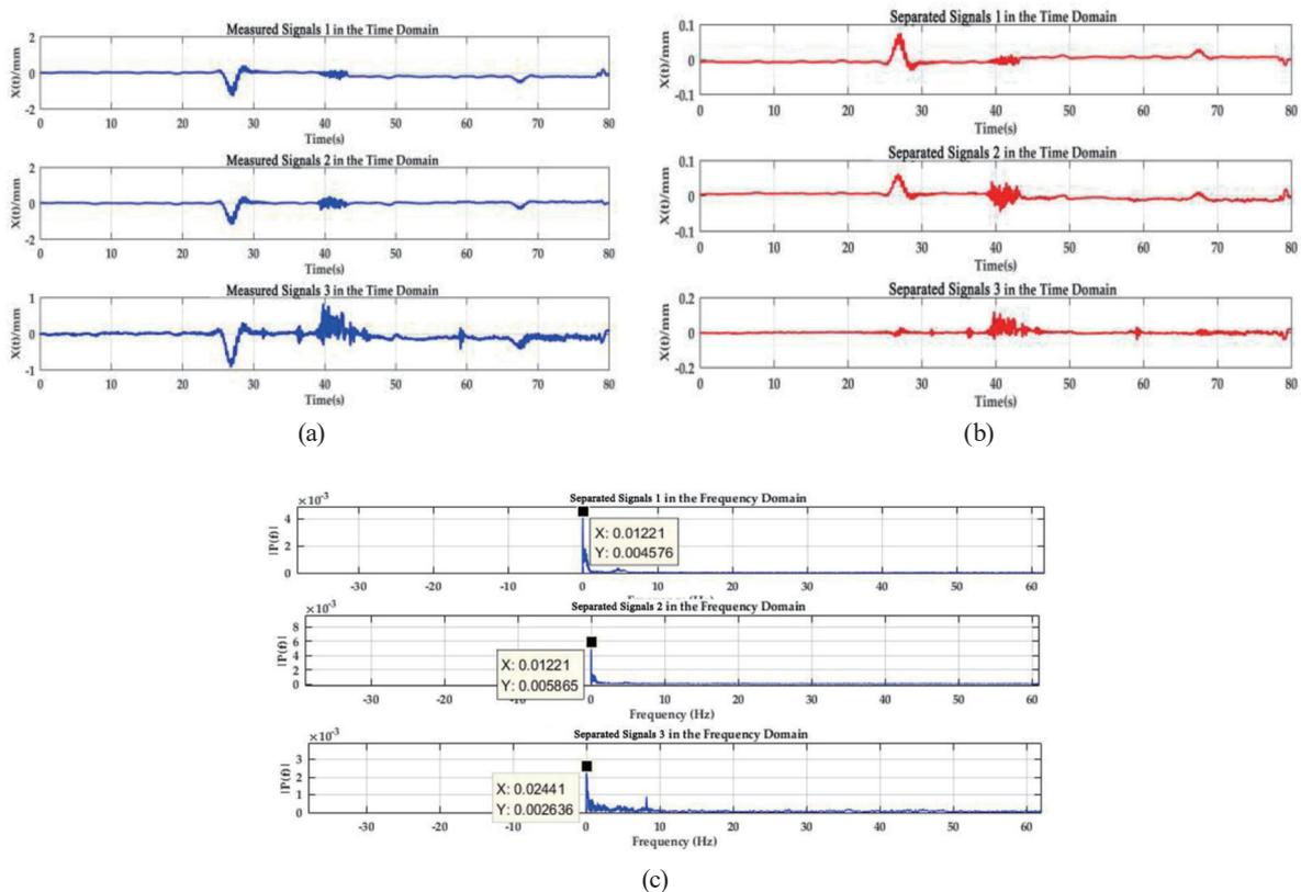
Fig. 8. (Color online) Signals of healthy bridge. (a) Measured signals. (b) Separated signals in time domain. (c) Separated signals in frequency domain.
