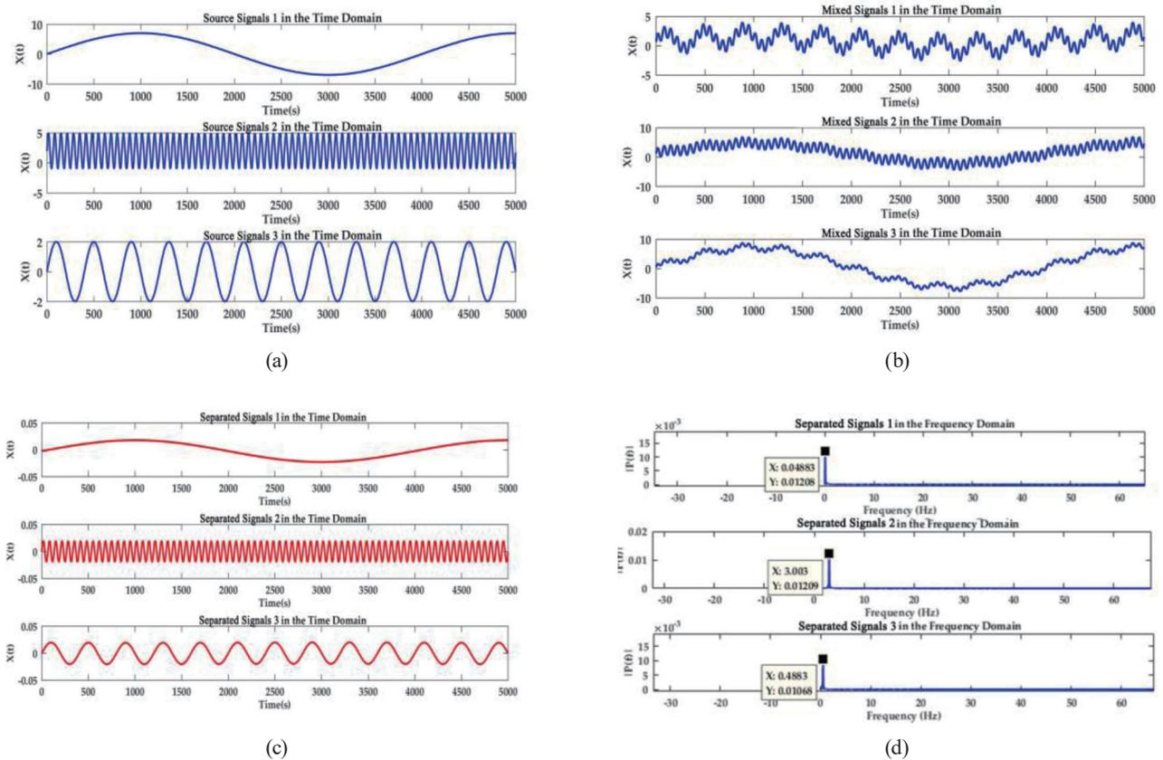
Fig. 5. (Color online) Simulation experiment 1. (a) Source signals in time domain. (b) Mixed signals in time domain. (c) Separated signal in time domain. (d) Frequency domain signals in time domain.
