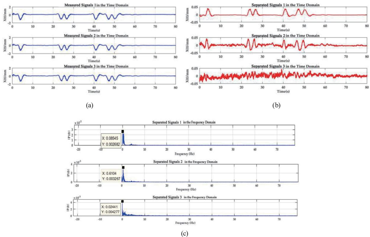
Fig. 7. (Color online) Signals of damaged bridge. (a) Measured signals. (b) Separated signals in time domain. (c) Separated signals in frequency domain.
