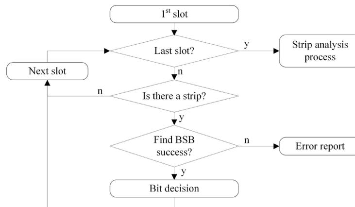
Fig. 1. Barcode recognition process.
