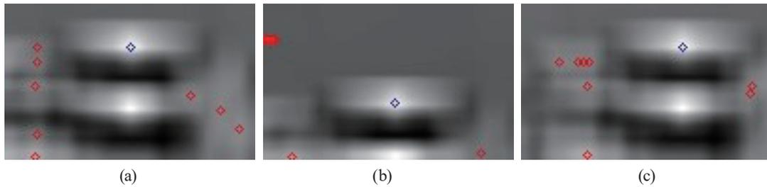
Fig. 9. (Color online) Examples of false peaks (red marks) that can be mistaken for the BSB peak (blue mark).
