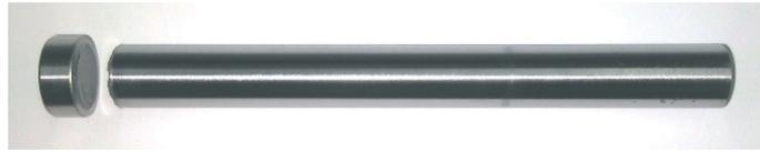
Fig. 7. Fracture of stepped circular punch.
