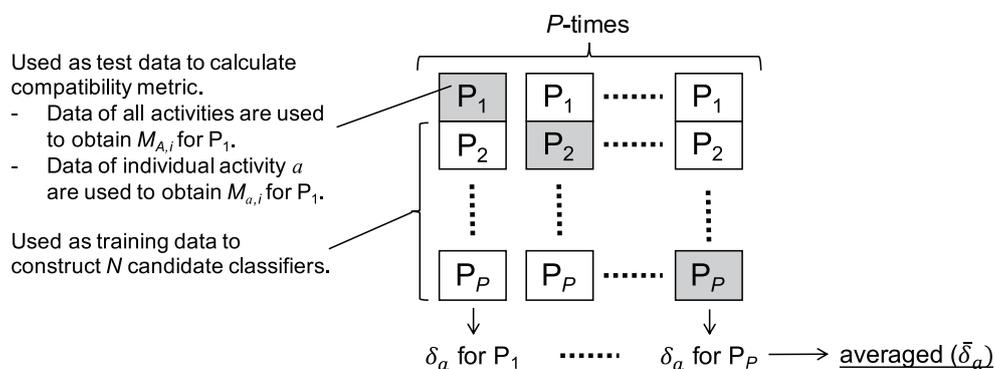
Fig. 3. LOPO-CV scheme for calculating the metric of effectiveness of particular activity ( $\delta_a$ ).
