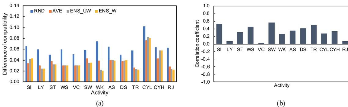
Fig. 6. (Color online) Effectiveness of individual activity in DaLiAc dataset: (a) difference-based and (b) correlation-based approaches. Note that in the difference-based method, a smaller value indicates a more effective activity, while in the correlation-based method, a larger value indicates a greater effectiveness.
