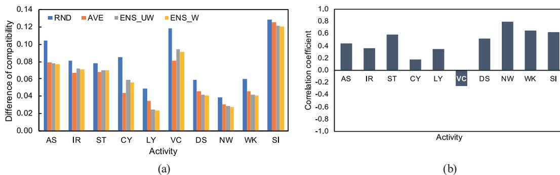
Fig. 5. (Color online) Effectiveness of individual activity in PAMAP2 dataset: (a) difference-based and (b) correlation-based approaches. Note that, in the difference-based method, a smaller value indicates a more effective activity, while in the correlation-based method, a larger value indicates a greater effectiveness.
