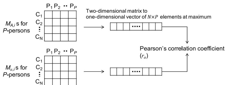
Fig. 4. Scheme for calculating Pearson's correlation coefficient ( $r_a$ ) between the compatibility obtained using the data of all activities ( $M_{A,i}$ ) and that obtained using the data of a particular activity  $a$  ( $M_{a,i}$ ).
