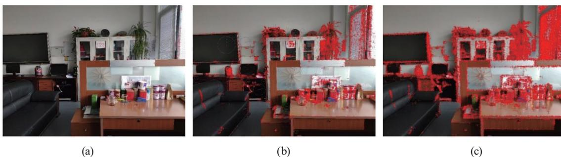
Fig. 6. (Color online) Results of feature point detection: (a) ORB, (b) SURF, and (c) SIFT.
