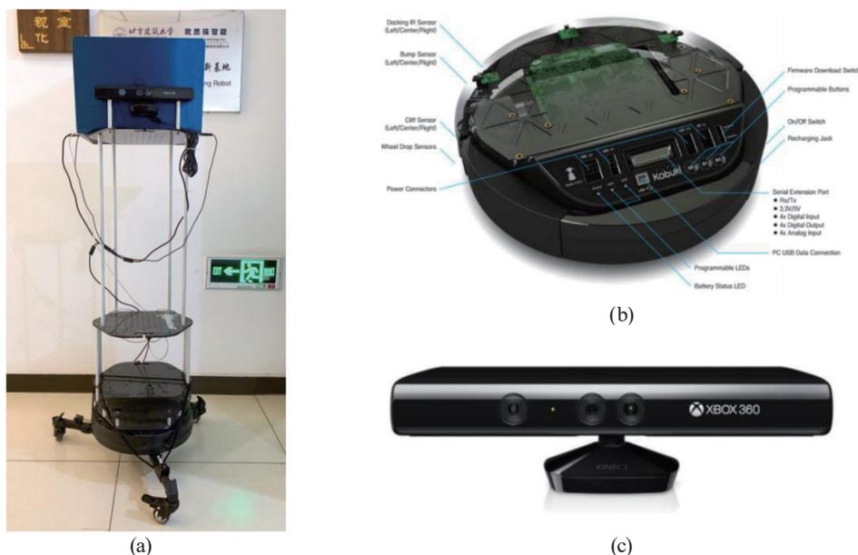
Fig. 4. (Color online) (a) RGB-D SLAM experimental platform, (b) Kobuki mobile base, and (c) Kinect V1 vision sensor.
