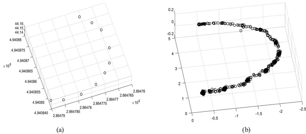
Fig. 10. (a) Distribution map of total station measurement points and (b) VO track.
