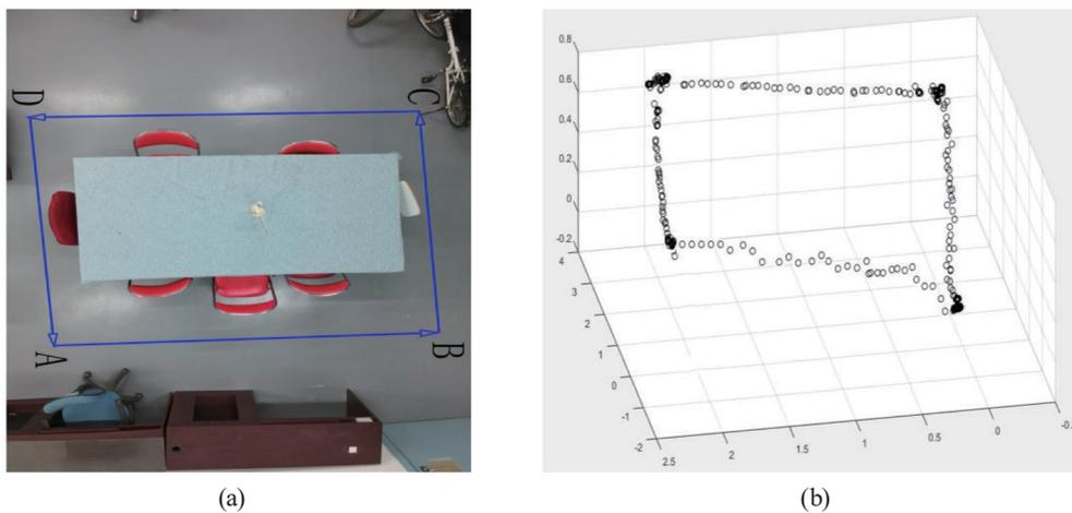
Fig. 11. (a) Closed-loop motion experiment environment and route and (b) VO track.
