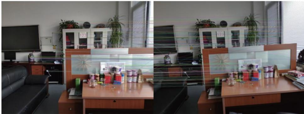
Fig. 7. (Color online) ORB feature matching using BF Matcher method.
