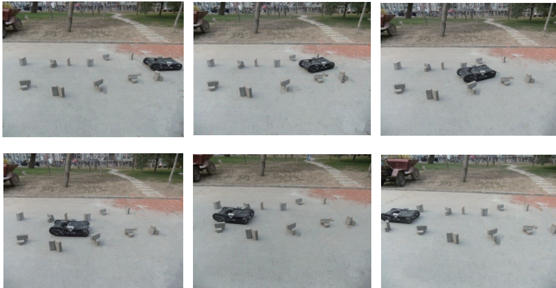
Fig. 6. (Color online) Experiment on robotic obstacle avoidance.
