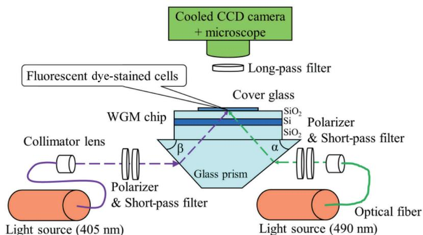
Fig. 1. (Color online) Optical setup of the parallel-incident-type WGM in this study.
