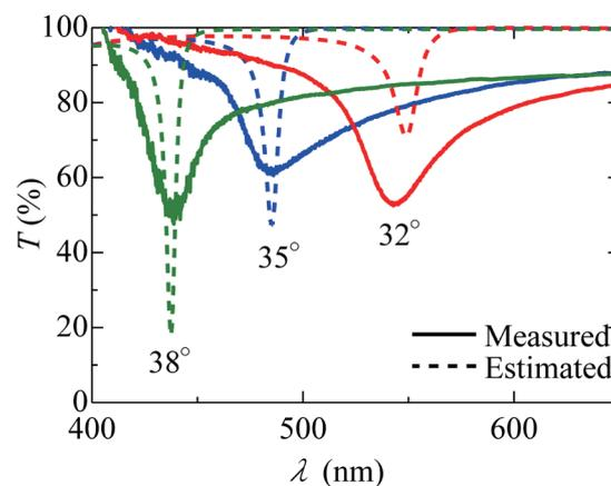
Fig. 2. (Color online) Reflectance spectra with WGM excitation when the base angles of the prisms were 32, 35, and 38°.
