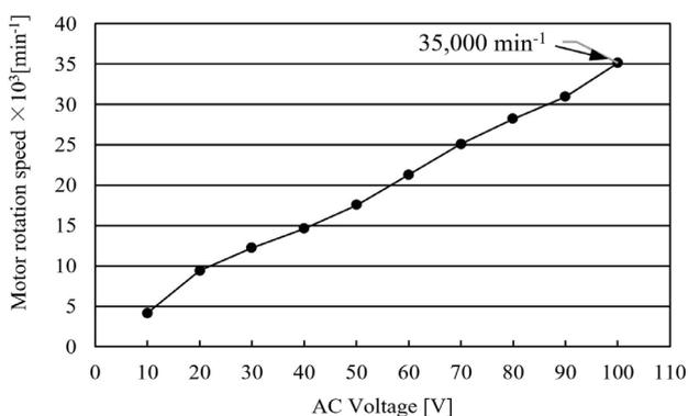
Fig. 3. Input voltage and rotation speed of motor.
