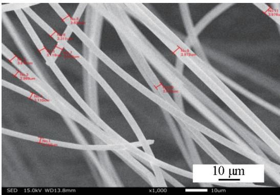
Fig. 12. (Color online) Enlarged SEM image of PP microfibers shown in Fig. 11.
