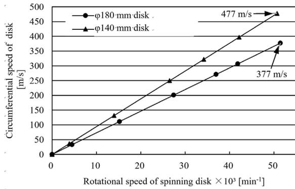
Fig. 5. Rotation and circumferential speed of disk.
