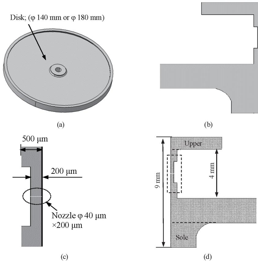
Fig. 2. Structure of the disk. (a) Top view of fiber-spinning disk, (b) detailed view of the disk, (c) enlarged view of the nozzle, and (d) cross-sectional view of the disk.
