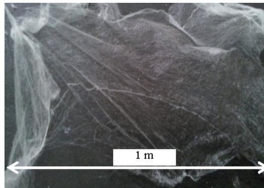
Fig. 13. Top view of microfibers (average diameter:  $1.9 \mu\text{m}$ ) melt spun at 86000 G for 2 min (Disk temperature:  $200 \text{ }^\circ\text{C}$ ).
