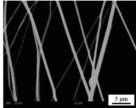
Fig. 15. Perspective view of nanofiber (average diameter: 595 nm) melt spun at 259000G (circumferential disk speed of 477 m/s) for 5 min.
