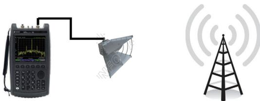
Fig. 1. (Color online) Experimental setup of ambient RF measurements.
