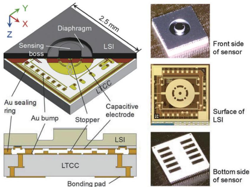
Fig. 2. (Color online) Integrated tactile sensor using sensor platform LSI flip-chip-bonded with LTCC substrate.<sup>(4)</sup>
