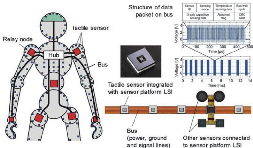
Fig. 1. (Color online) Bus-networked tactile sensor for robots.
