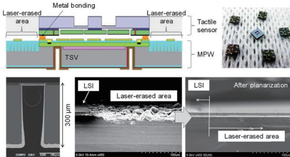
Fig. 3. (Color online) Integrated tactile sensor using sensor platform LSI with TSVs.<sup>(9,10)</sup>
