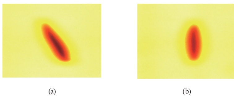
Fig. 12. (Color online) Backlit images of upright paddy seeds. (a) Upright red and (b) upright normal paddy seeds.
