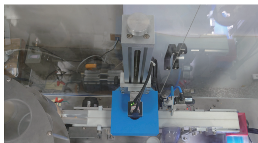
Fig. 18. (Color online) Top view of light-transmitting feeding system.
