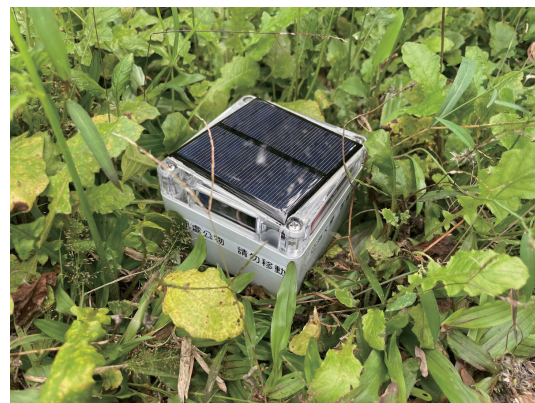
Fig. 9. (Color online) Soil humidity sensor and its module.
