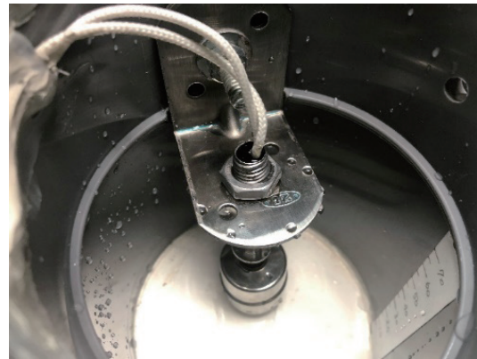
Fig. 6. (Color online) Magnetic sensor in water jar to measure amount of precipitation in micro-weather station.
