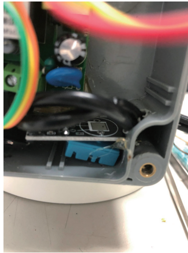
Fig. 7. (Color online) DHT11 module (blue box) connected with soil temperature sensor (black circuit with small LCS) module.
