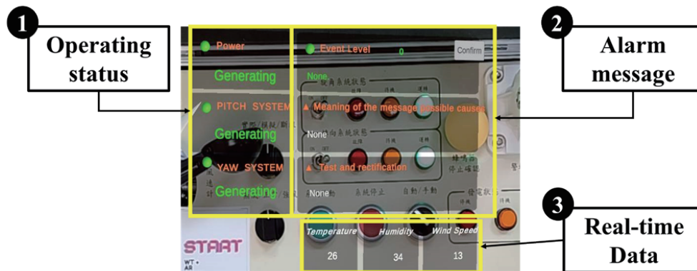
Fig. 6. (Color online) Wind turbine's normal operation screen display on AR device.
