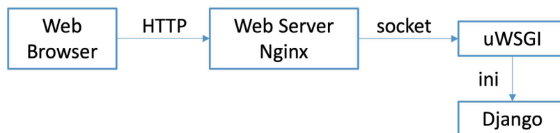
Fig. 4. (Color online) Forwarding process from Nginx web server to Django framework.
