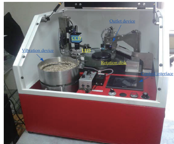
Fig. 8. (Color online) Autosorting system for PB and FB.
