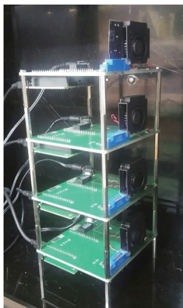
Fig. 2. (Color online) Setup of the four chip-controllers.
